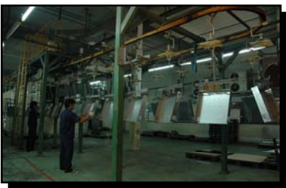
LINE CONVEYOR PAINTING
